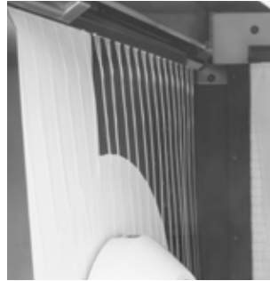
Flushing nozzle system
